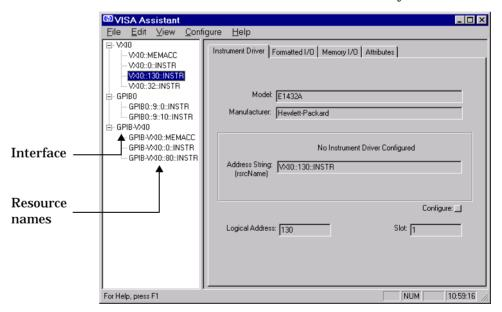
The VXIO::MEMACC and GPIB-VXIO::MEMACC resource names are associated with register-based communication. The Instrument Control Toolbox does not directly support these resource names. Instead, register-based communication is supported for VXI instruments with the memread, memwrite, mempoke, and mempeek functions, which are described in "Register-Based Communication" on page 4-13.
