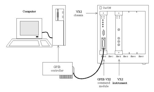
The GPIB-VXI interface is supported through a VISA-GPIB-VXI object. The features associated with a VISA-GPIB-VXI object are similar to the features associated with GPIB and VISA-VXI objects. Therefore, only functions and properties that are unique to VISA's GPIB-VXI interface are discussed in this section. These unique features are associated with:
