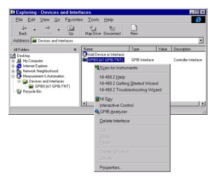
By selecting **Scan for Instruments** in the drop-down menu, you can display all instruments that are powered on and connected to the GPIB board. As shown below, a Tektronix TDS 210 oscilloscope with primary address 1 and a Hewlett-Packard 34970A data acquisition/switch unit with primary address 2 are connected and powered.
