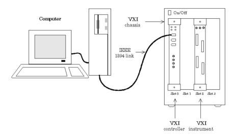
The VXI interface is supported through a VISA-VXI object. Many of the features associated with a VISA-VXI object are similar to the features associated with other instrument objects. Therefore, only functions and properties that are unique to VISA's VXI interface are discussed in this section. These unique features are associated with:
