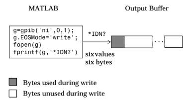
The \*IDN? command consists of six values since the End-Of-String character is written to the instrument, as specified by the EOSMode and EOSCharCode properties. Moreover, the default data format for the fprintf function specifies that one value corresponds to one byte.
