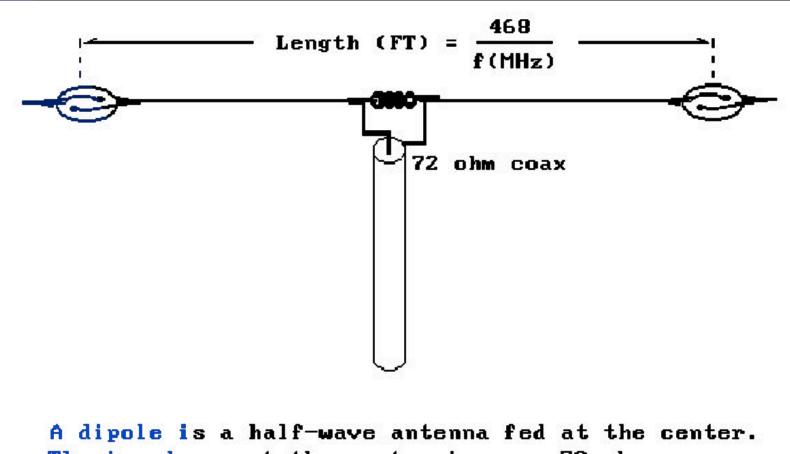
The impedance at the center is near 72 ohms.
