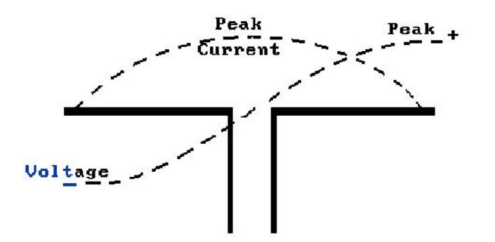
The basic dipole consists of two charges or elements which receive signals of opposite polarity.
