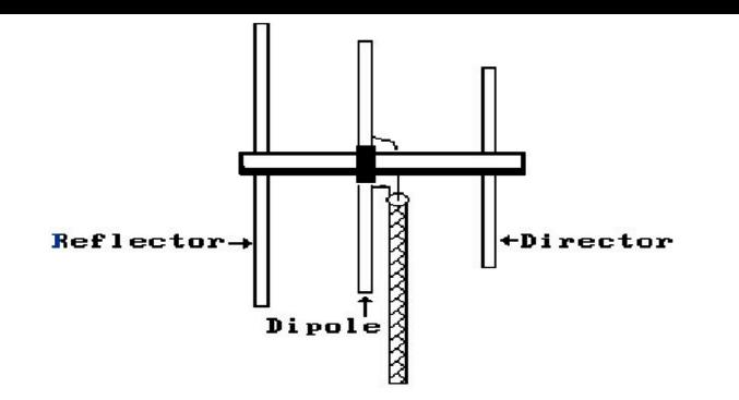
Adding a reflector and a parasitic element (director) to the dipole greatly improves its gain and directivity. Thus, the dipole becomes a "YAGI" antenna.
