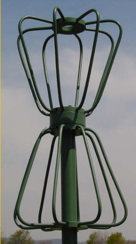
This new line of optimized wide bandwidth antennas provides a superior solution for communications, ESM, or measurement and testing systems requiring large instantaneous bandwidths with very flat impedance requirements in the VHF/UHF frequency range.
