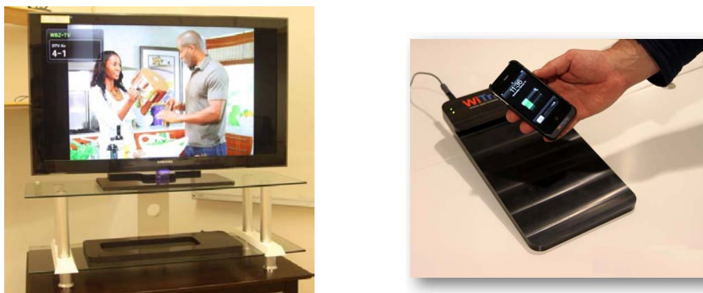
Figure 3: Photographs of magnetic resonance systems used to wirelessly power and operate an LCD TV (~250 W supplied wirelessly) (left) and to wirelessly charge a battery in a smart phone (~5 W supplied wirelessly) (right).
