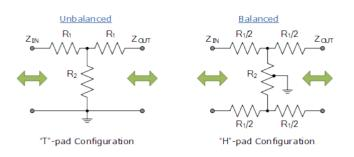
The **T-pad** Attenuator is so called because its configuration resembles the letter "T". The "T-pad Attenuator" is a symmetrical attenuator that can be used either for attenuation between equal impedances or impedance matching between unequal impedances. When the attenuation is high, the parallel shunt arm impedance becomes small. The balanced equivalent of the *T-pad attenuator* is called an **H-pad attenuator**.
