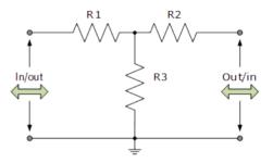
We can see that the T-pad attenuator is symmetrical in its design looking from either end and this type of attenuator design can be used to impedance match either equal or unequal transmission lines. Generally, resistors R1 and R2 are of the same value but when designed to operate between circuits of unequal impedance these two resistor can be of different values. In this instance the T-pad attenuator is often referred to as a "taper pad attenuator".
