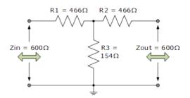
Then resistors R1 and R2 are equal to  $466\Omega$  and resistor R3 is equal to  $154\Omega$ , or the nearest preferred values. Again as before, we can produce standard tables for the values of the series and parallel impedances required to construct a  $50\Omega$ ,  $75\Omega$  or  $600\Omega$  symmetrical T-pad attenuator circuit as these values will always be the same regardless of application. The calculated values of resistors, R1, R2 and R3 are given below.
