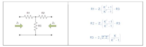
where: K is the impedance factor from the table above, and  $Z_1$  is the larger of the source/load impedances and  $Z_2$  is the smaller of the source/load impedances.
