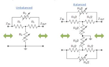
The **Bridged-T** Attenuator is variation on the standard T-pad design which has an additional resistive element forming a bridged network across the two series resistors and gains its name from the fact the input sources signal appears to "bridge" itself across the T-pad network without affecting the characteristic impedance of the circuit.
