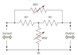
So for example above, if we wanted a variable bridged-T attenuator to operate on an  $8\Omega$  audio line with attenuation adjustable from -2dB to -20dB, we would need resistive values of:
