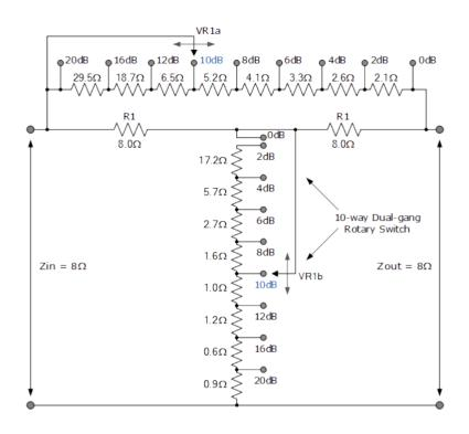
So for the bridging resistance set by VR1a at the -10dB point, the total resistance is equal to the sum of the individual resistances as is given as:
