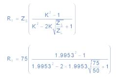
$R_{_1}$  = 75  $\times$  31.8 = 2,385  $\Omega$  (or 2.37  $k\Omega$  1%)
