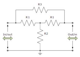
Resistor, R3 forms the bridge network across a standard T-pad attenuator. The two series resistors, R1 are chosen to equal the source/load line impedance. One major advantage of the bridged-T attenuator over its T-pad cousin, is that the bridged-T pad has a tendency to match itself to the transmissions lines characteristic impedance.
