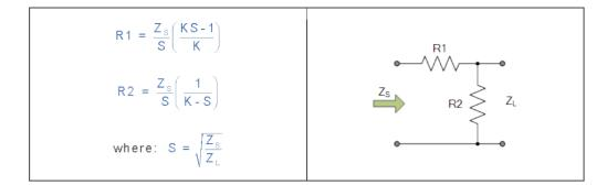
Between two unequal impedances, the impedance matching is towards the larger of the two impedances from the load.
