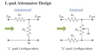
The **L-pad Attenuator** is the simplest attenuator design consisting of only two resistive elements and is more commonly known as a voltage divider circuit. The *L-pad attenuator* is an unbalanced asymmetrical attenuator circuit that can only impedance match in one direction. The balanced equivalent of the "L-pad Attenuator" is called a **U-pad attenuator**.
