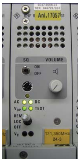
Figure II.7 Photograph showing details of one of the receivers in Fig. II.6. A power divider splits the signal picked up at the respective receiving antenna and feeds it to a buffer amplifier with a high large-signal immunity. A multiple-circuit preselector (Section III.11) located immediately behind the RX antenna socket relieves the subsequent stages. The operational quality by the depicted model EU231 from Rohde&Schwarz is so high that the unit must be tuned exactly to the receive channel. (Company photograph of Austro Control.)
