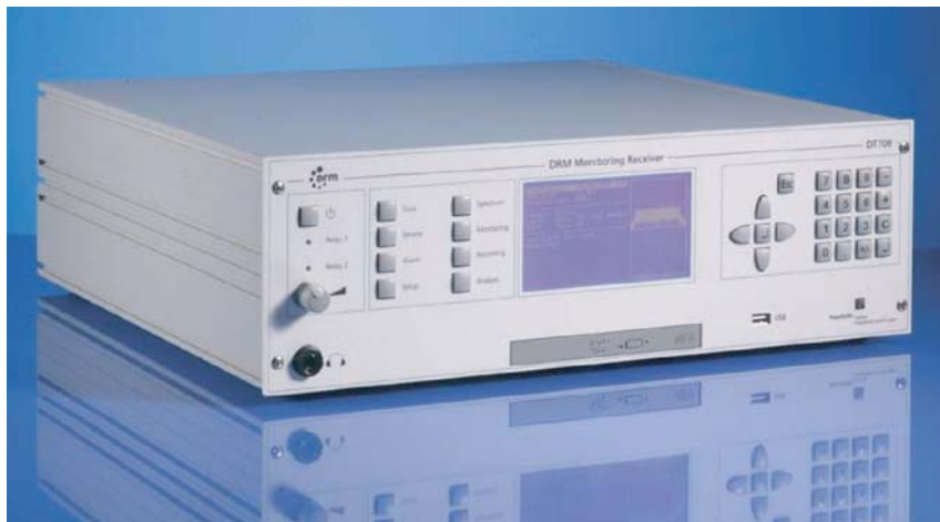
Figure II.47 DT700 professional audio broadcast receiver from the Fraunhofer Institute for Integrated Circuits, is used for low sound broadcasting bands ranging from 2,020 m to 11 m. The receiver enables the demodulation of AM, DRM (completely according to [44]), and SSB modulation types. The unit operates as a digital receiver of generation 2.5 (Fig. I.19), that is, as a quasi all-digital receiver. From an HF input level of -110 dBm the DRM signal is demodulated or decoded. Owing to its performance parameters this receiver is suitable for use as a control receiver to monitor transmit signals at DRM transmitter stations. (Company photograph of Fraunhofer Institute for Integrated Circuits.)
