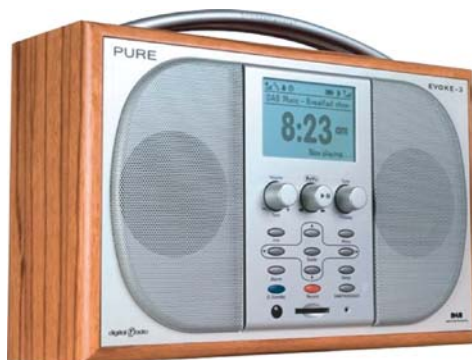
Figure II.46 EVOKE-3 audio broadcast receiver from PURE Digital, which allows DAB reception in the 1.5 m and 20 cm bands as well as analog VHF FM reception. The unit can stop and rewind the DAB program. This receiver can record audio programs over 30 hours on a 2 GB SD memory card. From an internal 6-line graphic display the electronic program guide for one week can be displayed in order to select audio programs for recording. (Company photograph of PURE Digital.)
