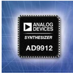
Figure I.9 Complete DDS capable of producing output signals up to 400 MHz with a resolution of 14 bits. Only a reference clock and a low-pass filter must be provided externally. (Company photograph of Analog Devices.)
