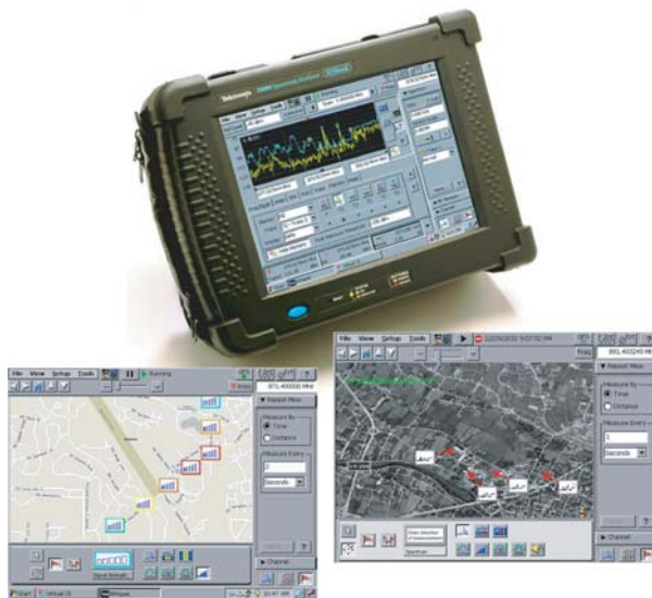
Figure II.40 The H500 RFHawk spectrum analyzer from Tektronix, together with a separate antenna, is specifically optimized for local signal tracking. The user interface allows superimposing local maps of the surroundings. By means of a GPS-based protocol [9] the device documents its own movements and provides a graphic display of the signal levels of the emission to be localized, measured at different locations. This allows detecting and avoiding faulty measurements taken at a certain location due to multiple signal propagation. The receiving frequency covers the range from 10 kHz up to 6.2 GHz. Maximum display width (span): 20 MHz; refresh rate of the spectral image: approximately 20 times per second; AM and FM demodulation. The dimensions are: 255 × 330 × 125 mm. (Company photograph of Tektronix.)
