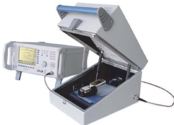
Figure III.3 The 4400 Mobile-Phone Tester from Aeroflex is a cost-effective multi-standard test platform for mass-market terminal equipment (GSM, HSCSD, GPRS, EDGE, CDMA2000, 1xEV-DO, WCDMA, TD-SCDMA). Standardized basic measurements on receiver modules are performed largely automatically via the air interface in compliance with the applicable standard. The specimen (mobile terminal equipment) is simply placed into the test well and the necessary connections are made automatically. (Company photograph of Aeroflex.)
