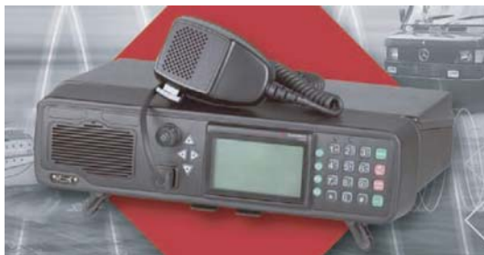
Figure II.11 Modern transceiver (radio equipment) TELCOR R125F from Telefunken Radio Communication Systems for wireless wide-area communication designed for voice radio, telefax and data traffic in the emission class J3E with 125 W. Within the entire received frequency range from 0.1 MHz to 30 MHz (1.6 MHz to 30 MHz transmission) up to 200 communication channels can be programmed in compliance with channel assignments. As an option, a GPS receiver can be integrated in the housing, enabling the operator to determine and transmit his own location without problems. (Company photograph of Telefunken Radio Communication Systems.)
