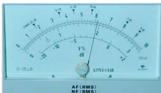
Figure III.18 Close-up view of the scale of a SINAD meter. For tuning purposes, analog displays often enable a more efficient workflow.
