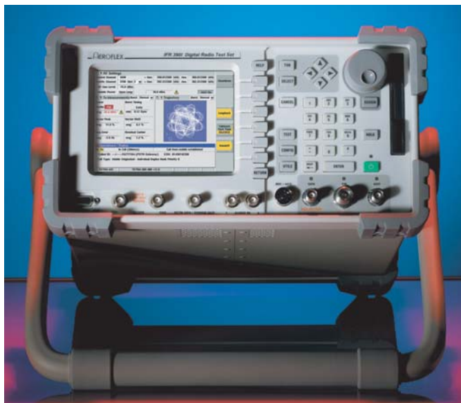
Figure III.2 The IFR39xx from Aeroflex belongs to a measuring station family of the latest generation. Owing to its modular design it can be configured for standardized TETRA receiver measurements. The unit also provides options for testing the basic parameters of radio receivers for AM and FM demodulation. (Company photograph of Aeroflex.)
