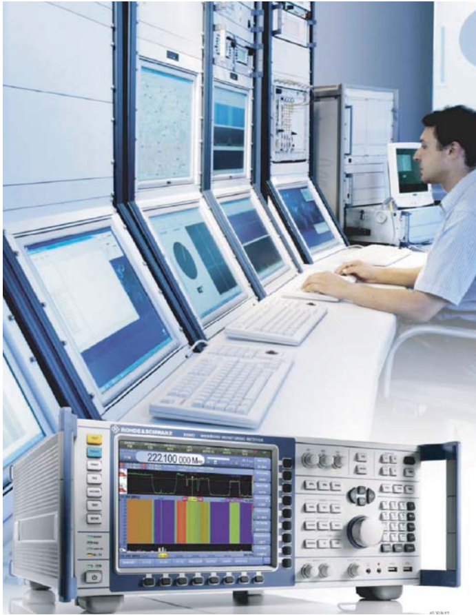
Figure II.13 ESMD compact wideband monitoring receiver from Rohde&Schwarz. It forms the centrepiece of a modern radio intelligence station comprising a search receiver, analysis receiver and a wide range of multi-channel demodulation capabilities. The unit can be upgraded for single-channel direction-finding. Fully equipped, it covers a receive frequency range from 9 kHz to 26.5 GHz. Performance data include: Maximum real-time bandwidth of 80 MHz, spectral image build-up with gap-free dynamically overlapping FFT; AM, CW, FM, PM, ISB, SSB, PULSE, analog TV, and IQ demodulation. The dimensions are 426 \times 176 \times 450 mm. (Company photograph of Rohde&Schwarz.)
