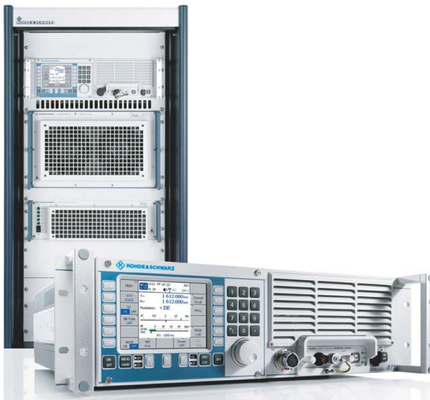
Figure II.10 Equipment family of the M3SR 4100 series from Rohde&Schwarz includes the model EK4100, a state-of-the-art receiver. Also available are transceivers with 150 W, 500 W or 1 kW HF transmit power (the rack in the background shows the 1 kW HF transmit stage and the required power supply unit). The units form a platform [10] that can be flexibly configured and upgraded via software. They are used by various classical conventional radio services as well as by the military. (When communicating on short waves one does not rely on telephone networks or cellular radio. HF communication equipment is comparatively easy to install and operates reliably. This applies particularly to areas of weak infrastructure or in emergency or natural disaster scenarios.)
