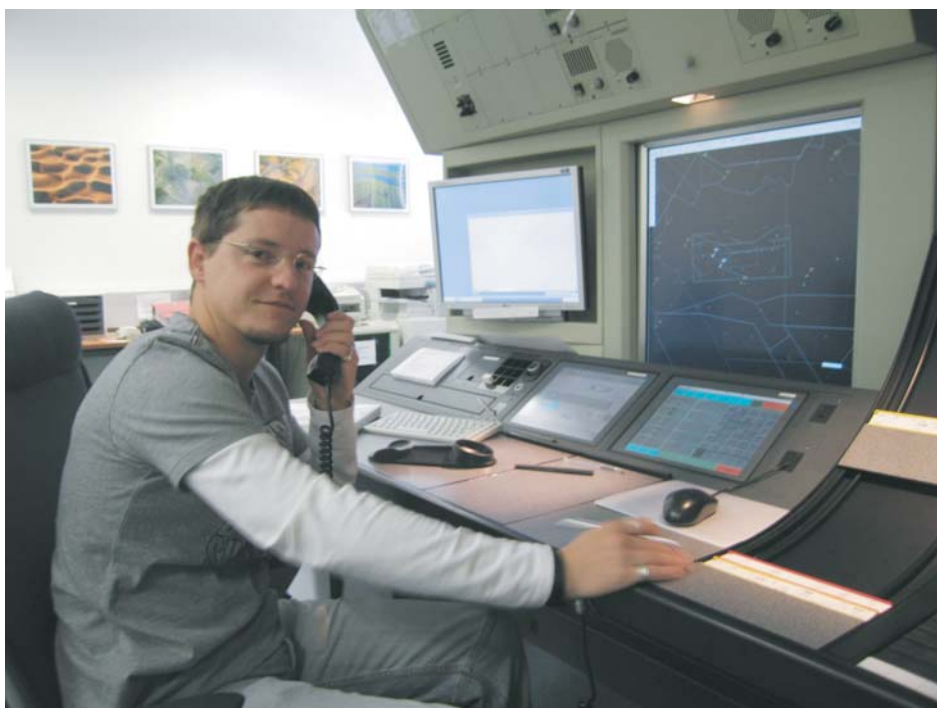
Figure II.43 A synthetically generated radar image for the head of air traffic control also includes DF information. The demodulated AF signal from one of the A3E voice radio receivers shown in Fig. II.6 is also inserted. (Company photograph of Austro Control.)
