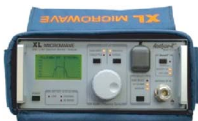
Figure II.42 The 2261A Analyze-R™ so-called Spectrum Monitor/Analyzer from Pendulum Instruments is primarily intended to detect local interferences in license-free and commonly used frequency bands (Table II.1). In combination with a GPS and external software it allows the documentation (logging) of receive levels and signal-to-noise ratios of signals received at various locations. With this method, the service coverage of a field station or one under construction can be tested. Receiving frequency range: 890 MHz to 940 MHz, 2.4 GHz to 2.5 GHz, 3.4 GHz to 4.2 GHz, 4.9 GHz to 6 GHz; display width (span): 100 MHz with 1 MHz resolution; refresh rate of spectral image: approximately 3 times per second; no demodulation capability. The dimensions are 89 \times 213 \times 333 mm. (Company photograph of Pendulum Instruments.)
