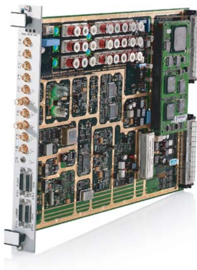
Figure II.26 EM010 receiver module on VXI basis from Rohde&Schwarz used as a functional element in a modern surveillance system. It may be used for hand-off reception or for technical analysis in the AMMOS radio intelligence system from the same manufacturer. It can be operated in parallel with several other receive paths. Performance data include: receive frequency range from 10 kHz to 30 MHz (optionally 300 Hz to 60 kHz via another input); memory search run on up to 1,000 programmed channels; AM, CW, FM, ISB, and SSB demodulation. (Company photograph of Rohde&Schwarz.)
