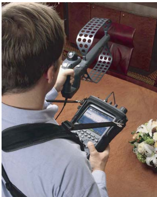
Figure II.41 HE300 hand-held direction finding antenna together with the PR100 portable monitoring receiver from Rohde&Schwarz. Four different antenna modules can be plugged, so the entire frequency range between 9 kHz and 7.5 GHz can be covered. Maximum display width (span): 10 MHz; refresh rate of the spectral image: 20 times per second; AM, CW, FM, ISB, SSB, PULSE and IQ demodulation. The dimensions are: 192 \times 320 \times 62 mm. (Company photograph of Rohde&Schwarz.)
