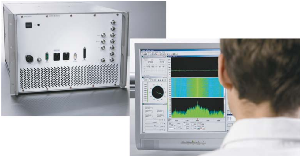
Figure II.38 The DFP 2400 compact VHF/UHF direction finding receiver (including DF processor and operating/display software) from PLATH. The device is intended for a frequency range from 20 MHz to 3 GHz (optionally to 5.8 GHz) and can operate in accordance with the Watson-Watt principle or the interferometer principle, depending on the type of antennas used. It also allows TDMA signal bearings. The analog receive bandwidth is fixed to 20 MHz. For different broadband signals (Section II.4.1) several surveillance widths of 20 MHz to 800 MHz can be selected by automatic tuning and shifting of the ‘20 MHz window’ in combination with FFT. (Company photograph of PLATH.)
