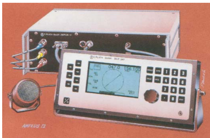
Figure II.45 AMPLUS 12 automatic three-channel direction finding receiver from PLATH (including DF processor and DF display unit), used predominantly in maritime and aeronautic traffic control with a frequency range of 108 MHz to 410 MHz. This type of equipment is employed in large numbers by the British Coast Guard. (Company photograph of PLATH.)
