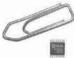
Figure II.50 MAS6179 integrated circuit for use in complete LW time signal receivers (here with sizes compared). This component offers the possibility to switch via a special input pin to three different transmitters. Additional external components required for its operation are only a ferrite antenna, three piezo-electric crystals for three different time signal frequencies, and a few capacitors. (Company photograph of MICRO ANALOG SYSTEMS.)
