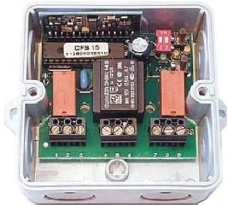
Figure II.4 Simple low-cost two-channel receiver for telecontrol purposes in the 35 cm ISM band. Two highly durable relays in the output circuit allow the potential-free shifting of the loads. Typical applications are wireless operation of garage doors, awnings, lights or fountains in ponds. For each output an automatic switch-off time can be programmed and random wire antennas are used. The systems are operated with a hand-held transmitter, the remote control. (Company photograph of RosyTec.)
