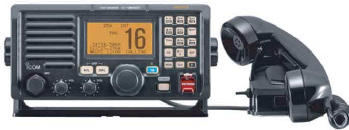
Figure II.8 Modern VHF transceiver IC-GM651 from ICOM for radio communication in commercial maritime traffic designed for voice radio in class F3E emission with 25 W. During operation on any channel a built-in independent receiver monitors the DSC channel 70 continuously (in class G2B emission). This allows automated emergency communication. Distress alarm messages received can be forwarded to coastal stations. An optional hand-held unit offers comprehensible sound reproduction, even in noisy surroundings. The receiving range covers the range from 156 MHz to 163.425 MHz (and the transmit frequency from 156 MHz to 161.450 MHz). (Company photograph of ICOM.)
