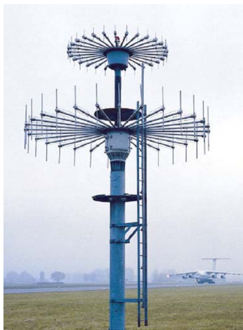
Figure II.44 Antennas of a Doppler direction finder for air traffic control. Two systems are arranged above one another in order to obtain sufficient DF sensitivity in the frequency range monitored.
