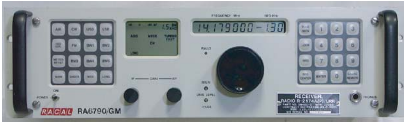
Figure II.9 Front view of a typical sturdy VLF/HF receiver meeting the highest demands in regard to both receiver characteristics (Part III) and electromechanical properties. The photo shows the RA6790/GM from RACAL, designed as a multi-conversion superhet (Section I.2.2) with fully analog signal processing. The easily rotating flywheel control to the right of the centre is for manual station search. The unit can be equipped with up to seven different IF filters and, at the same time, functions as an all-wave receiver featuring a receiving frequency range from 500 Hz to 30 MHz for AM, CW, FM, ISB (optional) and SSB demodulation. This unit is a 3 HE 19" plug-in module.
