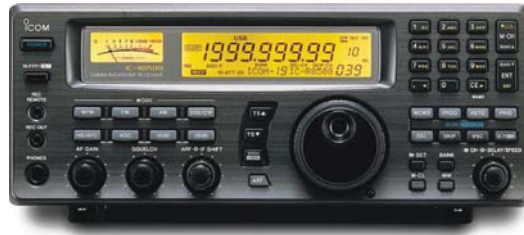
Figure II.25 IC-R8500 semi-professional broadband communications receiver from ICOM optimized for manually varying the tuned-in frequency. A recorder for registering the signals received can be connected to the REC or REC-Remote sockets on the front panel. The unit allows different query modes like skip memory, auto-storage and selective emission class search run. Performance data include: receive frequency range from 100 kHz to 2 GHz (>1 GHz with limitations); memory search run on up to 1000 programmed channels with a moderate search speed of 40 channels/s; AM, CW, FM, and SSB demodulation. The dimensions are 287 \times 112 \times 309 mm. (Company photograph of ICOM.)
