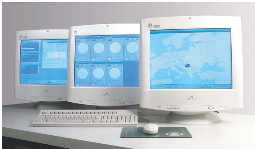
Figure II.39 Central control station for networks of several decentralized direction finders. The figure shows the OPAL system from PLATH as an example of an up-to-date workplace, showing (from left to right): The monitor for controlling the management tasks and for remotely controlling the field stations, the monitor for displaying the graphic results of the remote-controlled direction finders and the monitor for indicating the transmitter position. (Company photograph of PLATH.)
