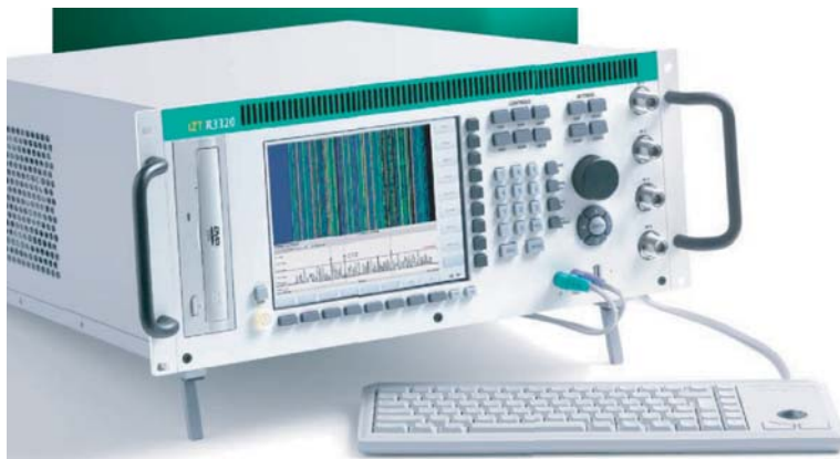
Figure II.14 R3320 modern short-wave surveillance receiver, from the Fraunhofer (research organization) spin-off Innovationszentrum für Telekommunikationstechnik. It functions as a digital receiver of generation 2.5 (Fig. I.19), i.e. quasi fully digital. Besides the real-time bandwidth of up to 24 MHz it allows FFT-based spectrum analysis with a frequency resolution of better than 2 Hz and the simultaneous demodulation of several received frequencies. Performance data include: Receive frequency range 9 kHz to 32 MHz, maximum real-time bandwidth 24 MHz (deactivated preselector, Section III.11), spectral image build-up with up to 1,000 FFTs per second, FM demodulation and IQ offline analysis, 19" plug-in module of 3HE. (Company photograph of Innovationszentrum für Telekommunikationstechnik.)
