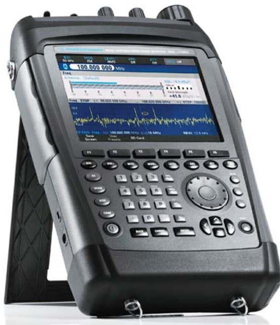
Figure I.33 PR100 allows continuous tuning for receiving in a frequency range from 9 kHz to 7.5 GHz with a noise figure (Section III.4.2) of less than 20 dB across the entire receive frequency range. The portable unit has a weight of 3.5 kg, including the battery pack (see Fig. II.41). Analysis of the received signals can also be carried out on the 6.5 inch colour display. Information can be stored on a built-in SD memory card without external accessories. For special applications all receiver functions can be remotely controlled via a LAN interface. The unit can be upgraded optionally for use as a single-channel direction finder in the range from 20 MHz to 6 GHz (Company photograph of Rohde&Schwarz).
