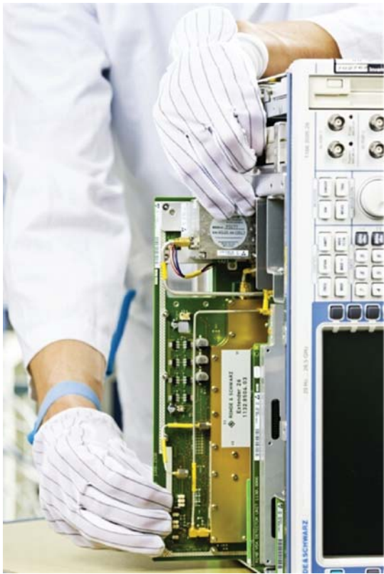
Figure II.2 Example of a service-friendly mechanical construction for a radio receiver with the individual circuit boards plugged into the chassis. (Company photograph of Rohde&Schwarz.)
