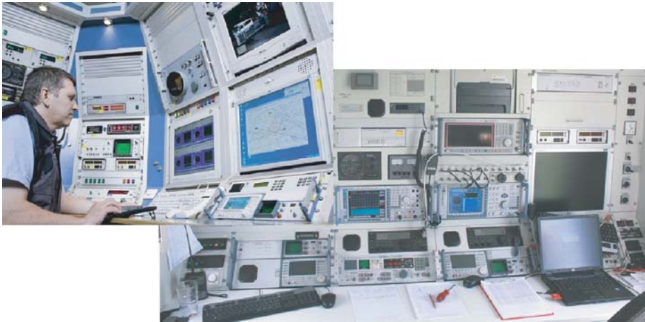
Figure IV.2 Analysis of the radio frequency spectrum following the ITU (International Telecommunication Union) guidelines in professional radio surveillance. During these procedures powerful receivers are subjected to practical daily operating situations and then pushed to their limits and beyond. (Company photograph of Federal Austrian Telecommunications Authority.)
