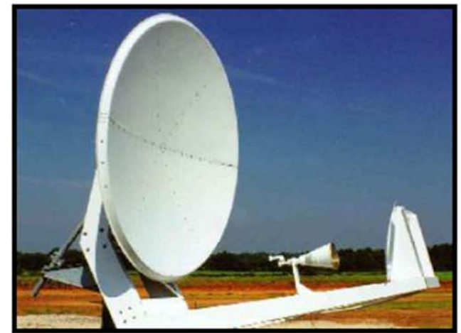
Dual Offset Reflector Antenna
