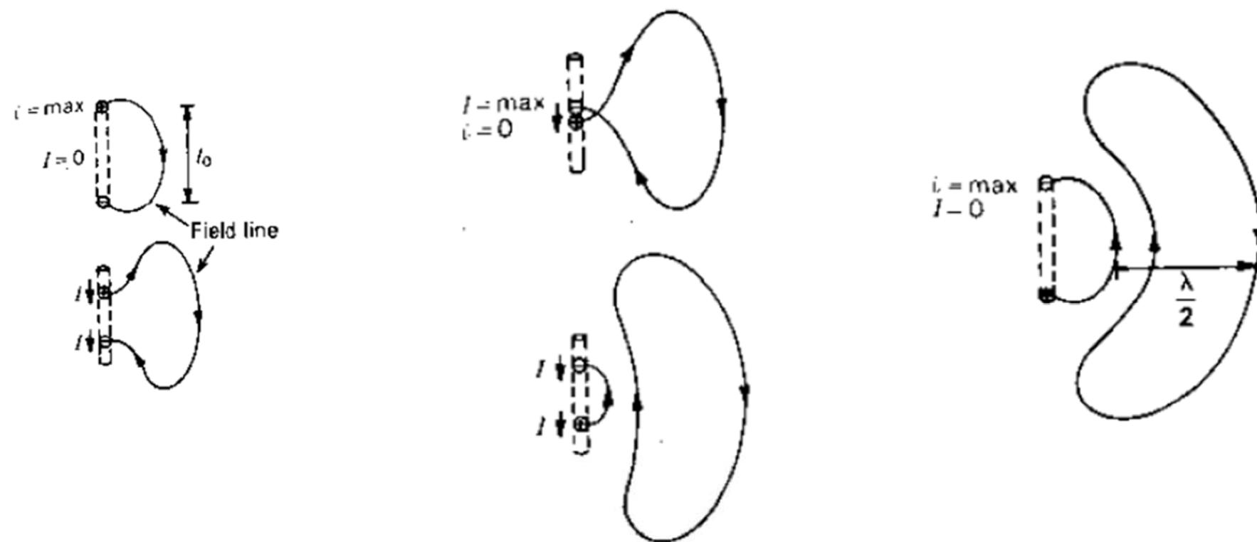
Oscillating electric dipole consisting of two electric charges in simple harmonic motion, showing propagation of an electric field line and its detachment (radiation) from the dipole
