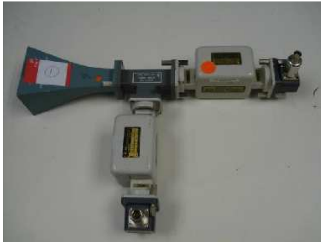
Figure 10.3: Setup for simple monostatic radar. Waveguide components include: horn antenna, ferrite isolators, H-plane (shunt) T-junction, coaxial-to-waveguide adapters and a diode detector (mixer). A CW microwave oscillator is used as the signal source, and an oscilloscope for viewing the output of the mixer.
