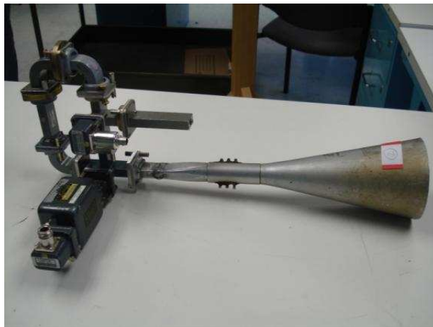
Figure 10.4: Setup for refined version of monostatic radar. Waveguide components include: horn antenna, ferrite isolator, magic tees, coaxial-to-waveguide adapters and a diode detector (mixer).
