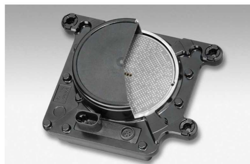
Fig. 4. Cross section and photograph (courtesy of Conti ADC) of a folded reflectarray antenna (frequency 76.5 GHz, antenna diameter 90 mm, depth 23 mm).
