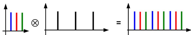
Fig. 10. Ideal antenna excitation distribution and convolution of transmit and receive antenna excitation resulting in a densely populated synthetic array.
