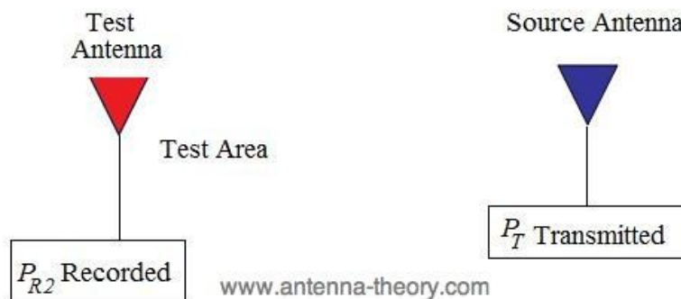
Figure 2. Record the received power with the test antenna (same source antenna).
