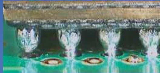
Formation of Solder Balls
