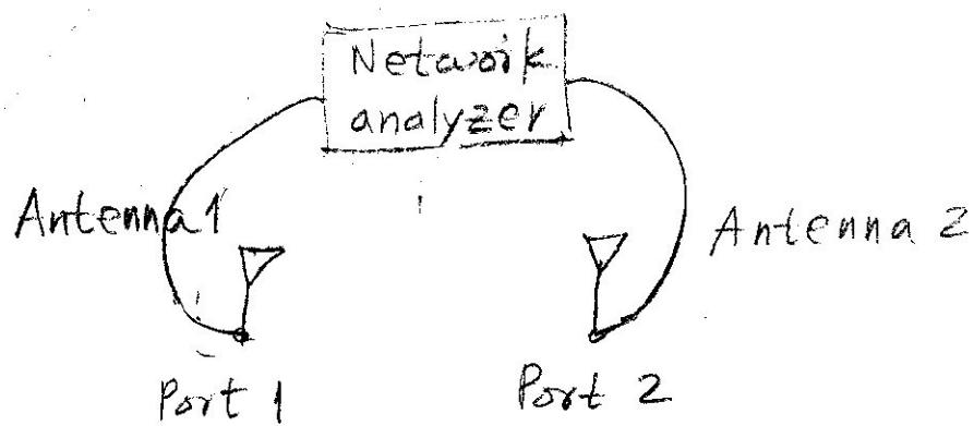
$$\text{Measure } [S] = \begin{bmatrix} S_{11} & S_{12} \\ S_{21} & S_{22} \end{bmatrix}$$
