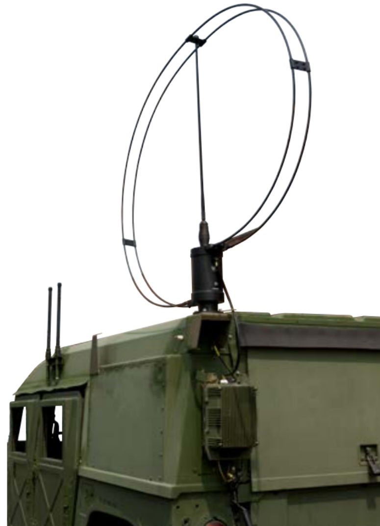
RF-3134-AT003/5 mounted on vehicle
