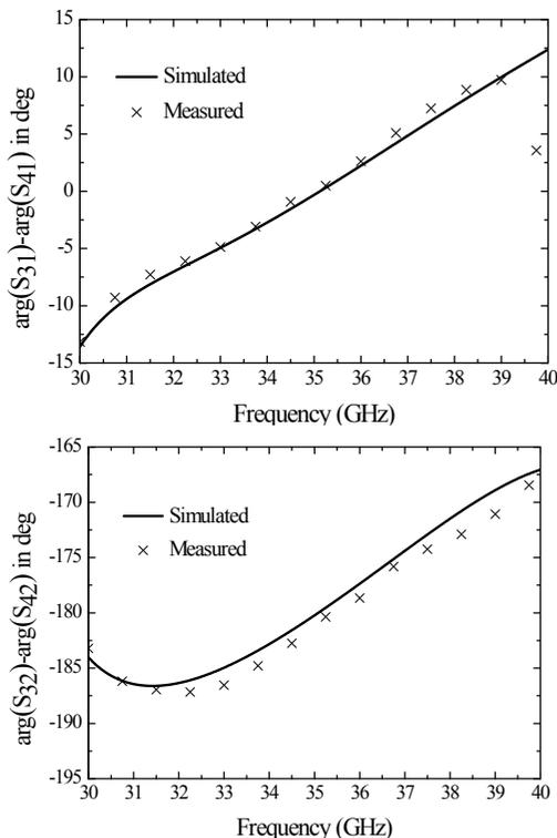
Fig. 6. Phases of the transmission coefficients between coupled ports of the fabricated ring hybrid coupler
