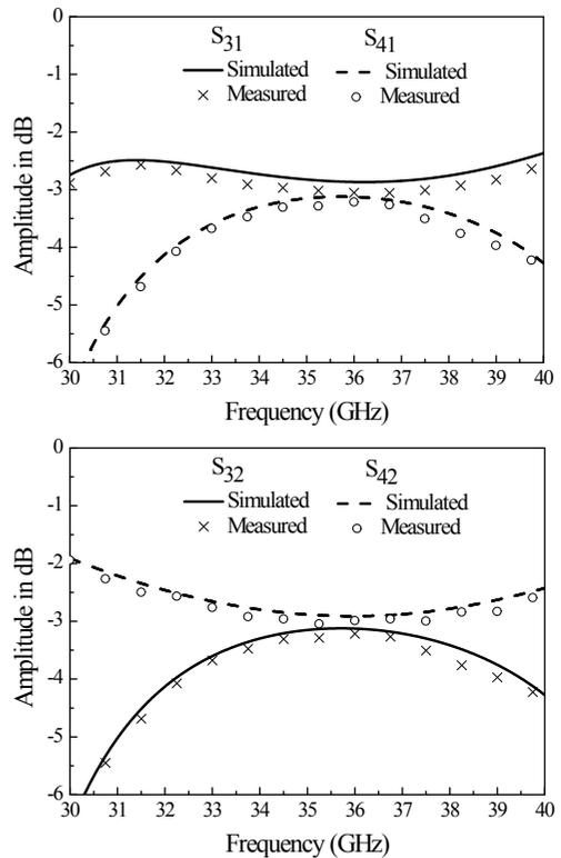
Fig. 5. Amplitudes of the transmission coefficients between coupled ports of the fabricated ring hybrid coupler
