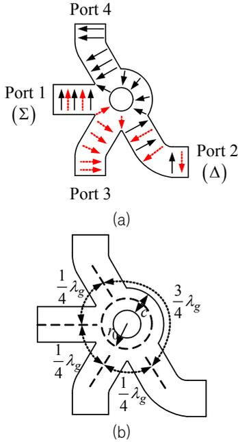
Fig. 1. (a) Reference directions of the electric field in the ring hybrid and (b) Nominal dimensions of the ring sections
