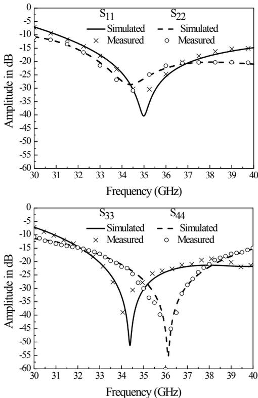
Fig. 3. Reflection coefficients of the fabricated ring hybrid coupler
