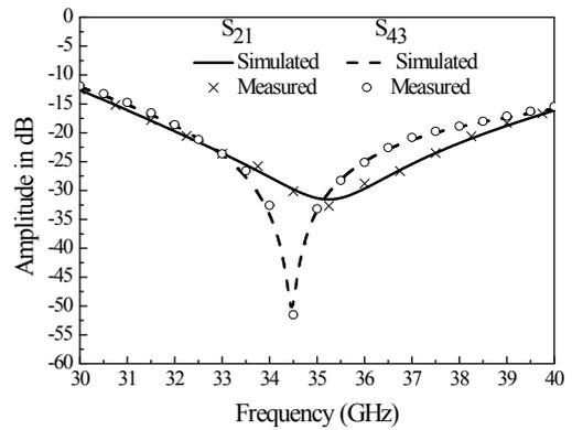
Fig. 4. Transmission coefficients between isolated ports of the fabricated ring hybrid coupler
