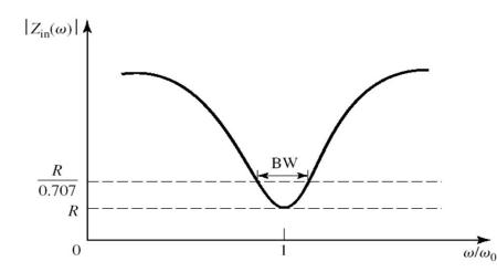
The input impedance magnitude versus frequency.
