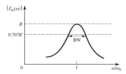
The input impedance magnitude versus frequency.
