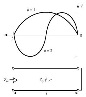
A short-circuited length of lossy transmission line and the voltage
