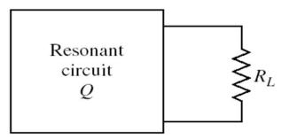
A resonant circuit connected to an external load,  $R_L$ .
