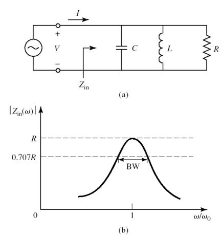
A parallel RLC resonator and its response. (*a*) The parallel RLC circuit. (*b*) The input impedance magnitude versus frequency.
