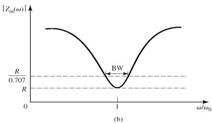
A series *RLC* resonator and its response. (*a*) The series RLC circuit. (*b*) The input impedance magnitude versus frequency. • The frequency in which
