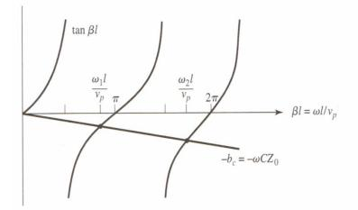
Solutions to (6.78) for the resonant frequencies of the gap-coupled microstrip resonator.
